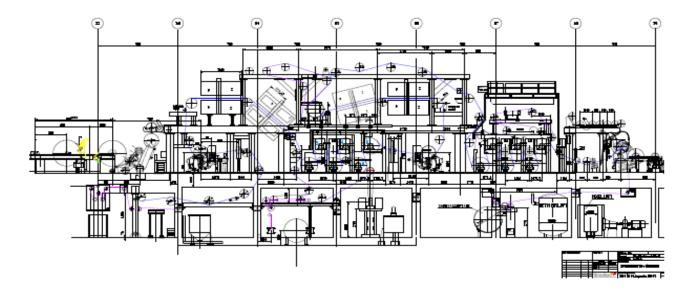
Operating speed 1,420 m/min, consisting of: Unwinding, coating unit 1, carbon blade coater (2015), hot air drying, cylinder contact drying, coating unit 2, manufactured by Voith/Sulzer, type Jetflow F, with Voith Web inspection system, Parsytec web monitoring system, Working speed max. 1,600 m/min, Infrared drying, cylinder contact drying, machine bonnet, manufactured by Voith/Kofra, reel, working width 7,500 mm
